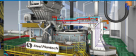
Next Generation Ecological and Economical Arc Furnace (ECOARC light™)
